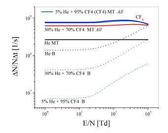
Figure 7.: Rate coefficients for  $He^+$  in  $He/CF_4$  mixtures as a function of E/N: momentum transfer.
