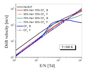
Figure 3.: Drift velocity for  $\mathrm{He^+}$  in  $\mathrm{He}/\mathrm{CF_4}$  mixtures as a function of  $\mathrm{E/N}.$
