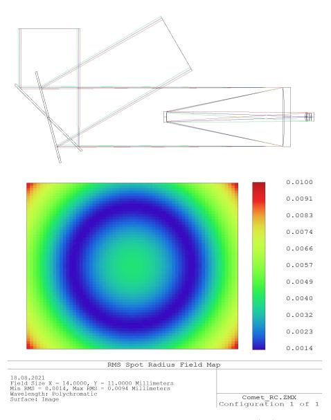
**Figure 1.** Optical scheme of the telescope with a repointing mirror (top), image quality (bottom).
