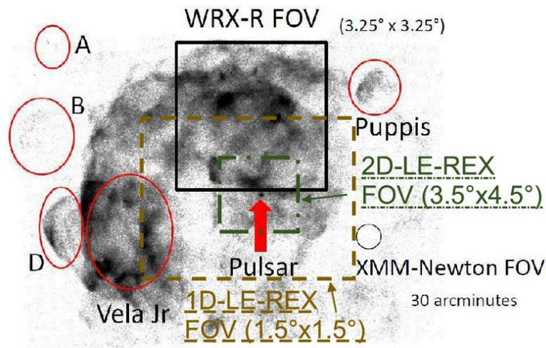
**Figure 2.** The field of view of all optics aboard the WRX-R compared to the FOV of XMM Newton (Dániel et al., 2017)
