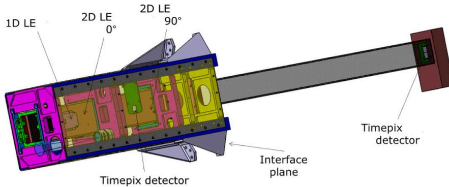
**Figure 1.** The arrangement of Hard X-ray payload
