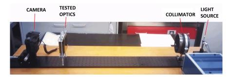
Figure 4. Experimental setup
