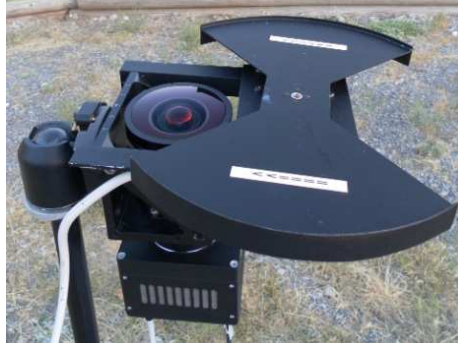
Figure 1. A SPOSH camera with a rotating shutter
