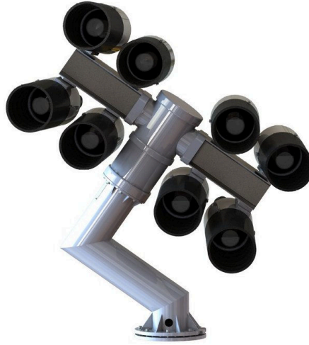
Figure 1. INF multiaperture telescope: 8 x VT-78d's on the ASA DDM160 mount.
