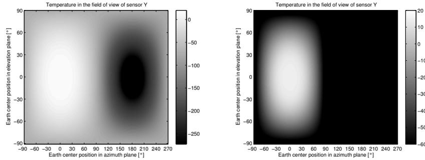
**Figure 5.** Low temperature threshold of sensors influences the range of angles in which the Earth surface temperature is detectable.
