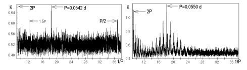
**Figure 3.** Left : Periodogram for the "early" superhump stage, JD 2455888–897. *Right* : The periodograms for the "ordinary" superhump stage, JD 2455899–906. The ordinate "K" is the inverse of the parameter  $\theta$ , calculated by the Lafler-Kinman method (Lafler & Kinman, 1965). The periods of superhumps and some harmonics are marked by arrows.
