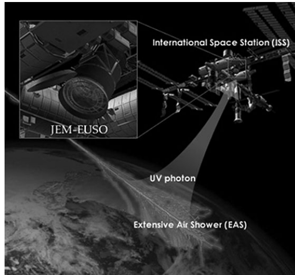
Figure 3. The planned location of the detector JEM-EUSO at the International Space Station (ISS - Kibo Exposed Facility).
