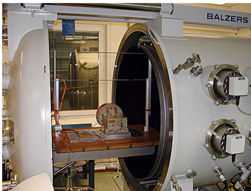
Figure 5. Thermal-vacuum testing of the NUADU detector in space environment simulator (IRF Kiruna, Sweden).
